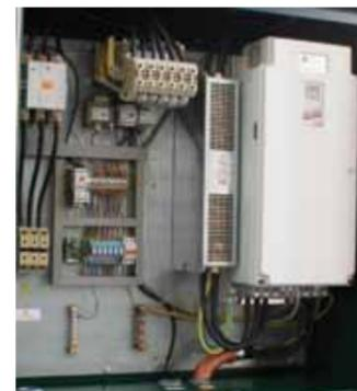
**ANTRIEB BEI VST-KOMPRESSOREN**
